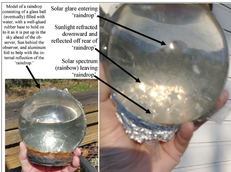
Fig. 3. A glass raindrop, backed by reflective foil, duplicates a raindrop making a spectrum (rainbow) of the Sun through refraction and reflection.
