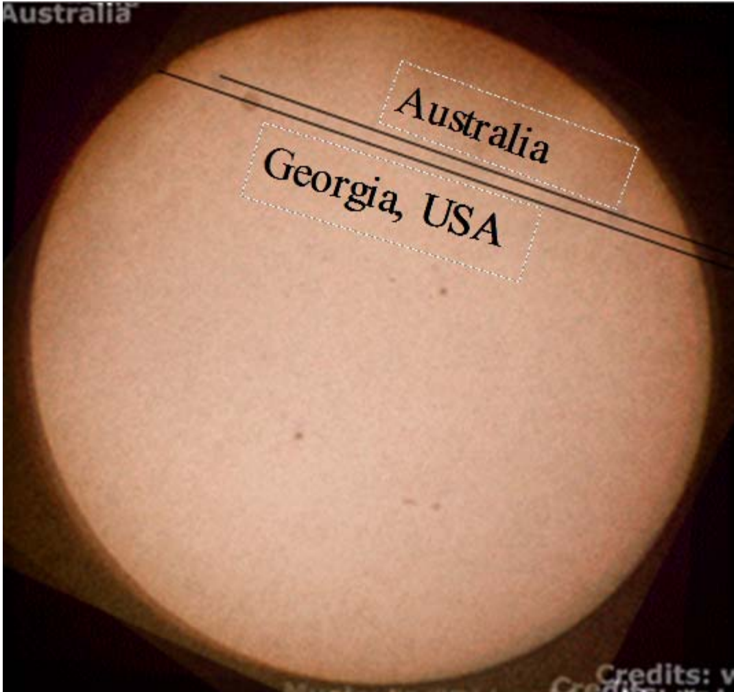
An image of all four Sun photos from Cairns and Marietta during the Transit of Venus with tracks drawn on the image.
