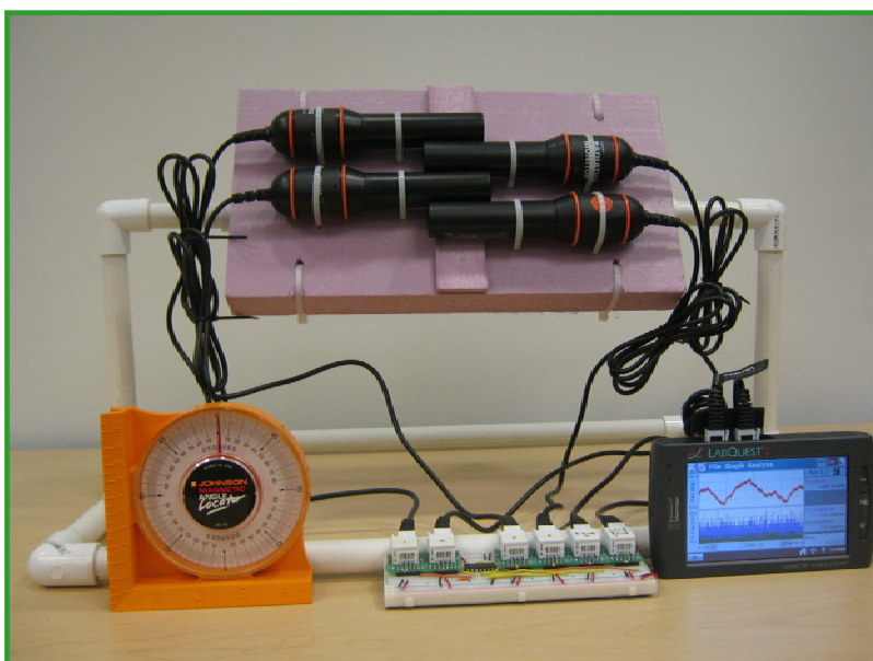
Figure 5. This design is built on a PVC pipe frame so that the detector can be pointed at different zenith angles Z . Using four instead of two radiation monitors allows us to vary the size of the solid angle seen by the detector and reduce the number of accidental coincidences. However, only two radiation monitors are needed to measure the zenith angle distribution of muons.
